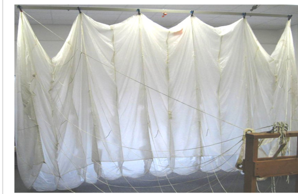
Hanging the canopy by the tail helps in both assembling and inspection.
